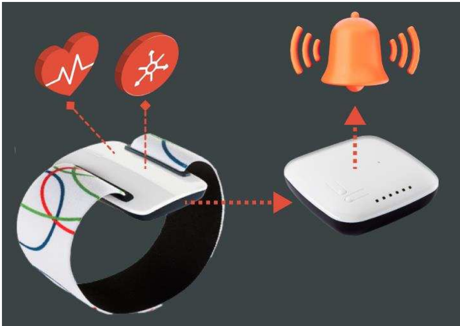
Figure 1 The NightWatch bracelet contains a photoplethysmographic heart rate module and a three-dimensional accelerometer. When a specific heart rate or movement threshold or pattern is detected, the algorithm triggers an alarm so caregivers can intervene. The signals or alarms are transmitted by Digital Enhanced Cordless Telecommunications Ultra Low Energy (DECT ULE) directly to the base, which may be connected to a local area network for further transmission of the data and alarms. DECT ULE is a wireless communication standard with greater range, reliability, and safety than Bluetooth or Wifi. Figure published with permission from LivAssured.
